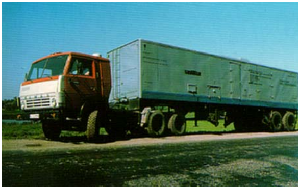
PAES-2500B mobile, automated, of tropical version, f = 60 Hz Series production since 1989
