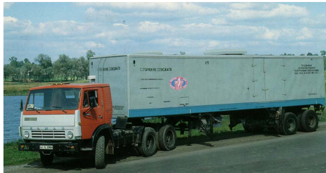
Base modification PAES-2500 mobile, automated, f = 50 Hz Series production since 1970
