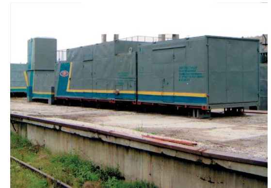
EG-2500 block-transportable modification, automated, f = 50 Hz Series production since 1993
